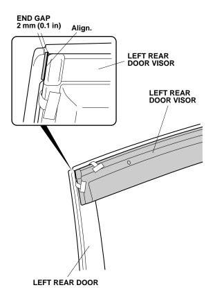
18. While applying light pressure against the left rear door visor, carefully remove the adhesive backings in the order shown. Use your fingers to push up each bracket so there is no gap between the brackets and the door sash.
