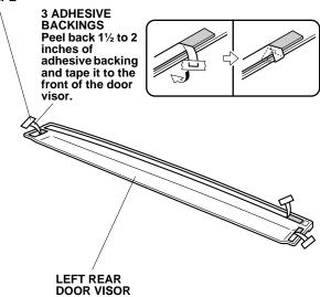
16. Align the clip holes in the left rear door visor with the bracket holes, and install the clips while pushing up on each bracket A. There should be no clearance between the brackets and the door sash. NOTE: Be sure the bracket and the door visor are aligned properly. Once the clip is installed, it cannot be reused.
