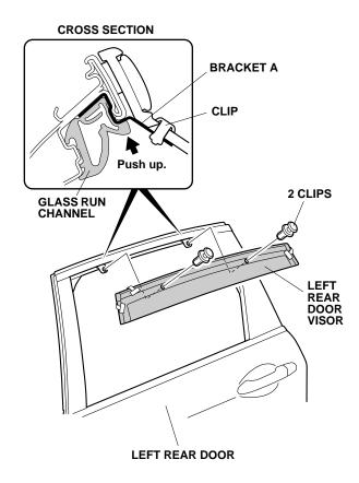
17. Adjust the end gap of the left rear door visor as shown.
